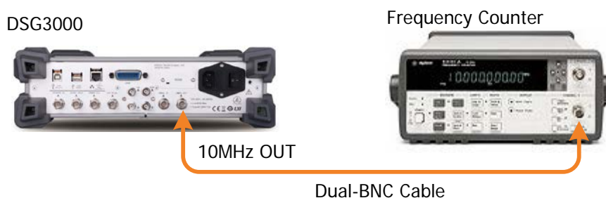
Figure 2-1 10 MHz Reference Output Accuracy Test Connection Diagram
